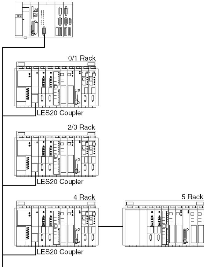
In the illustration above, the TSX Series 7 processor for the 0/1 rack was replaced by a TSX LES 20 coupler. A TSX LES 20 coupler was installed in position M of the 2/3 rack. The 2/3 rack is fitted with a power supply. These two couplers were connected to the I/O extension bus by two TSX LES 62 connector terminal blocks.
