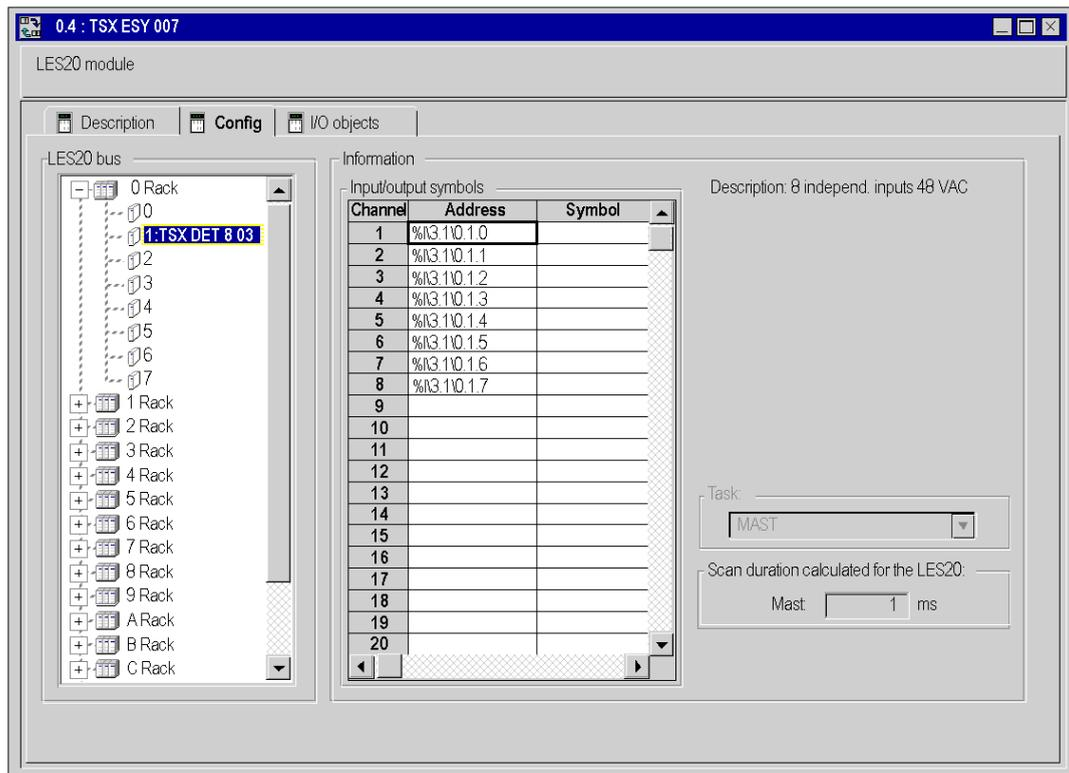
The front tab indicates the currently used mode (**Config** in this example). Each mode may be selected using the tab for the mode.
