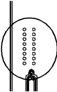
A green LED on indicates whether the corresponding TSX7 rack or one of its modules has a communication fault.
