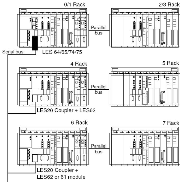
The TSX LES 20 Series 7 module manages data exchange with the TSX 7 CPU. It transforms the I/O data that it receives via serial bus into data on the parallel bus of the extension racks. Through a TSX LES 61/62 connection box, the LES20 Series 7 module has the address of the extension rack it manages.
